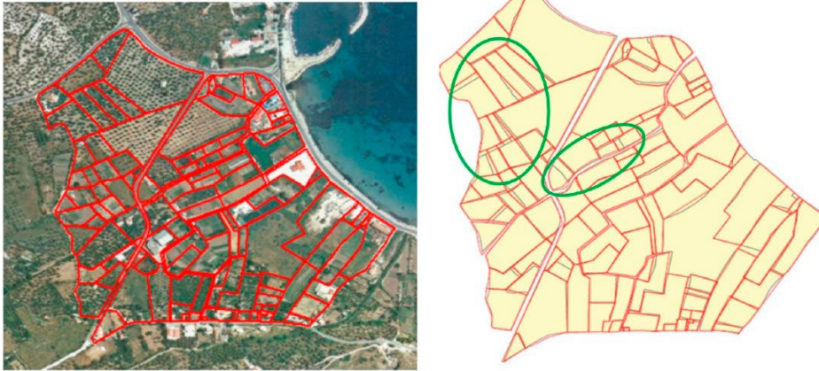
Figure 11: Left – digitized parcels in Greece; Right – comparison between polygons collected by volunteers (in red) and by surveyors (in blue). (Source: Apostolopoulos et al., 2018)
