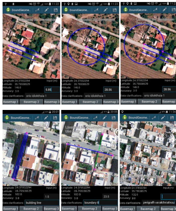
Figure 41: Examples of the use of BoundGeometry application to digitize hidden boundary corners.
