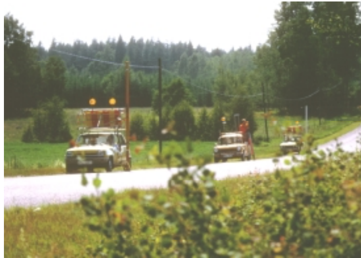
Fig 2. Setup with the motorised levelling technique.
