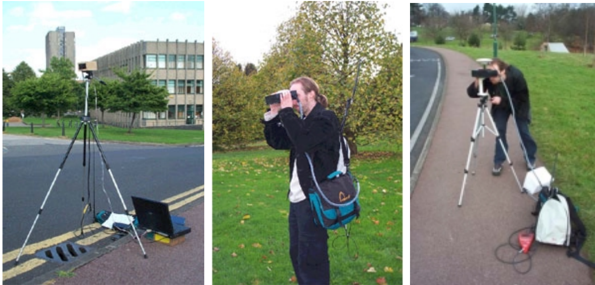
Figure 4 Camera and digital compass unit development. First trials (left), Working prototype (middle), Overcoming EMI problems (right).
