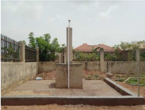
Figure 2: Tersus Smart AXE402 GNSS Antenna, SOGPOS Osun CORS in Osogbo (APPSN Osun State)
