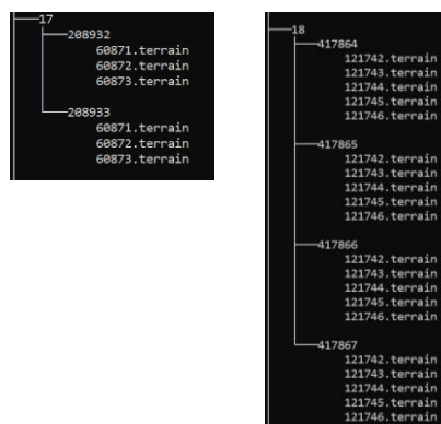
Figure 5. Tree structure of quantized-mesh format dataset for zoom level 17 and 18
