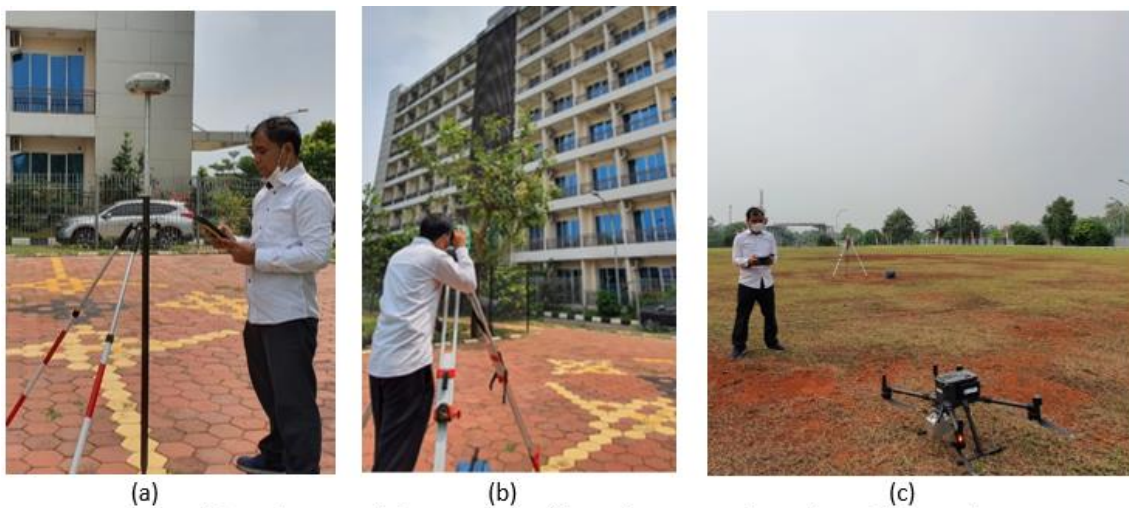
Field Work Image : (a) GNSS CORS, (b) Total Station Reflecterless, (c) UAV Lidar
