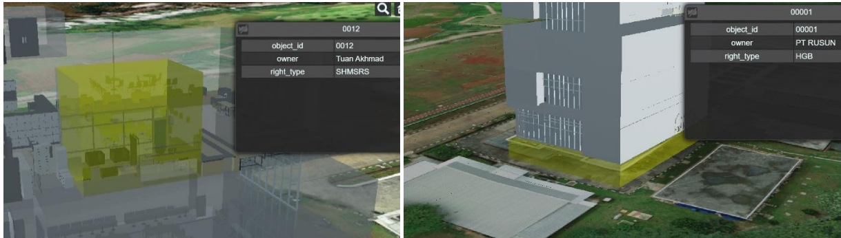
Figure 12. Access legal spaces information blocked by walls (left) and terrain (right) with transparency capability
