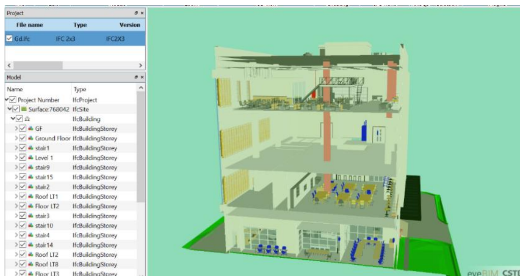
Figure 2. PUSDATIN MoASP/BPN BIM data displayed in eveBIM
