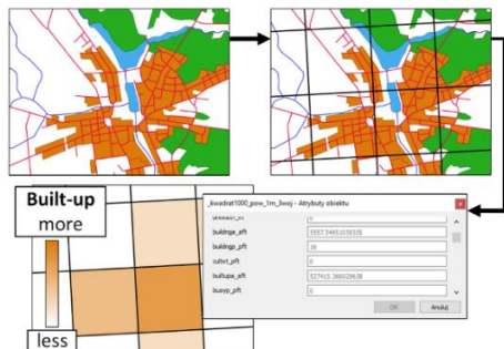
Fig. 2 Conversion of a vector model based on the example of the "built-up area" category.
