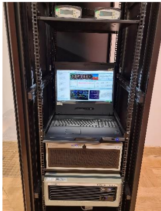
Figure 5. GNSS signal simulator (Spirent series GSS9000) (source: WUT-left and Spirent - right)
