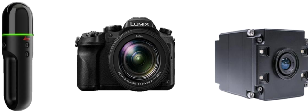
Figure 2: Sensors to be tested (from left to right): Leica BLK2GO [8], Lumix DMC-FZ2000 [9], Lucid Helios Time of Flight 3D camera [10]
