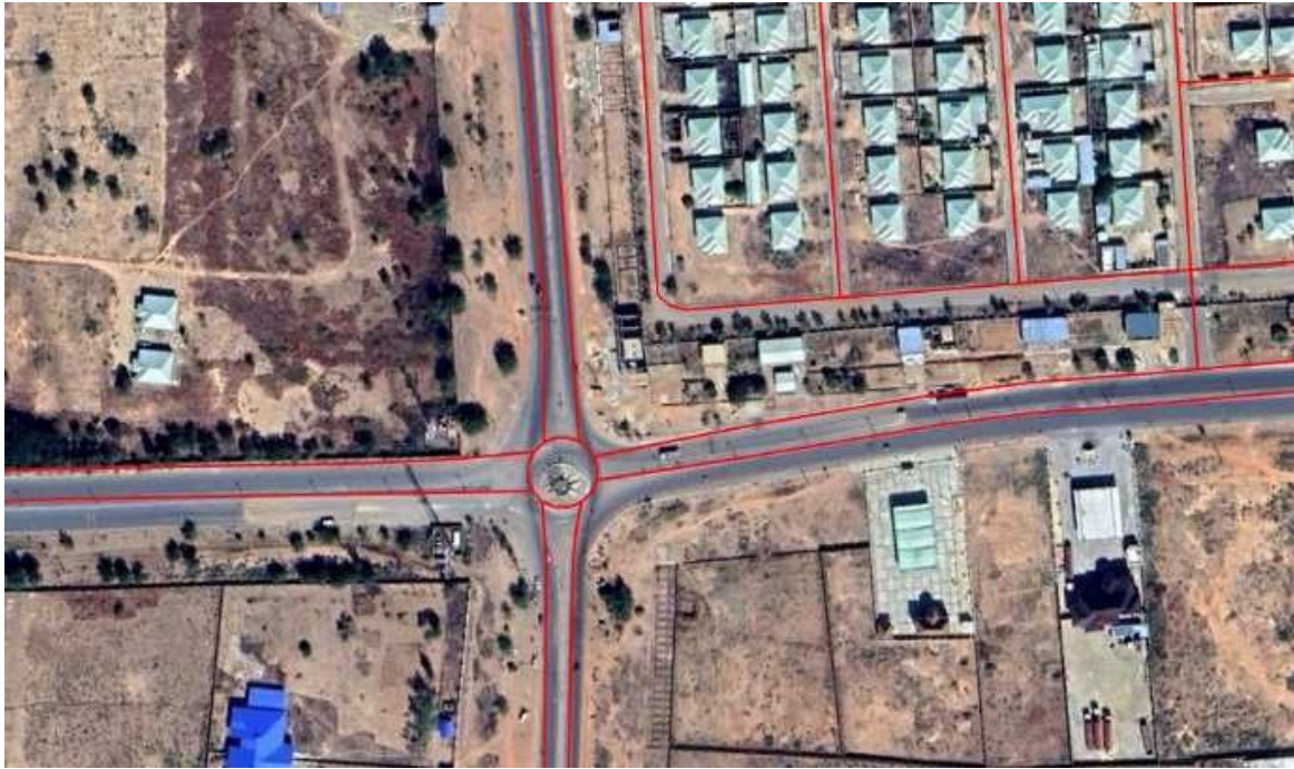
Plate 1 Overlaid OSM and Image of the area depicting OSM shift from the center
