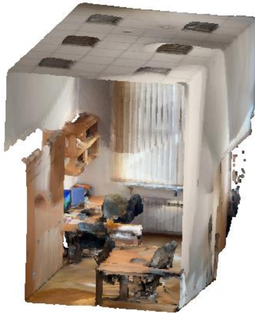
Figure 1 Colored point cloud view of the section of an office room scanned by the iPhone 13 Pro
