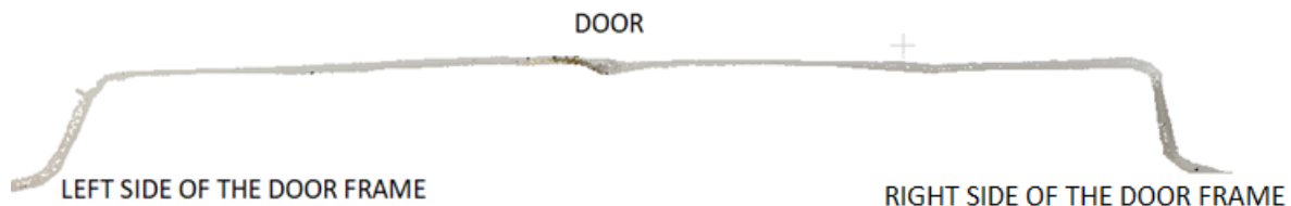
Figure 4. Horizontal section of a door frame scanned with iPhone 13 Pro
