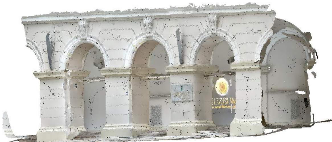
Figure 2 Colored point cloud of a fragment of the main hall of Warsaw University of Technology scanned by the iPhone 13 Pro
