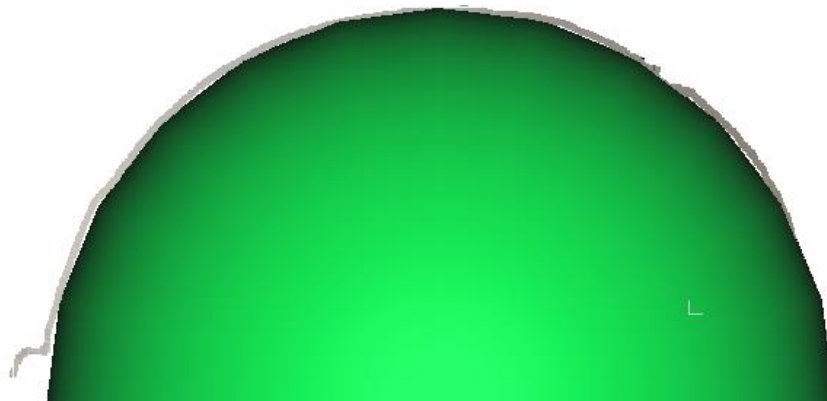
Figure 5. View of a fragment of the circle fitted into a cross-section of the point cloud from the iPhone 13 Pro representing an arch in the lintel of the cloisters of the main auditorium of Warsaw University of Technology
