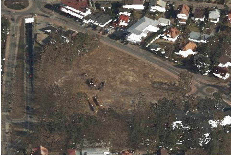
Figure 5. Colorized ALS point cloud from 2018, depiction of the area of the fire station in Legionowo.
