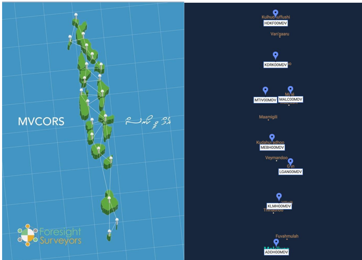
Figure 1 – Distribution of the MVCORS stations when the project has been fully completed (left) and current distribution of installed stations (right)
