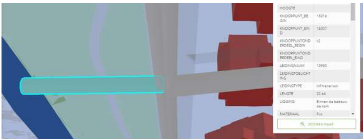
Figure 5. Open sewage locations data with additional attributes about the material, form, width etc.
