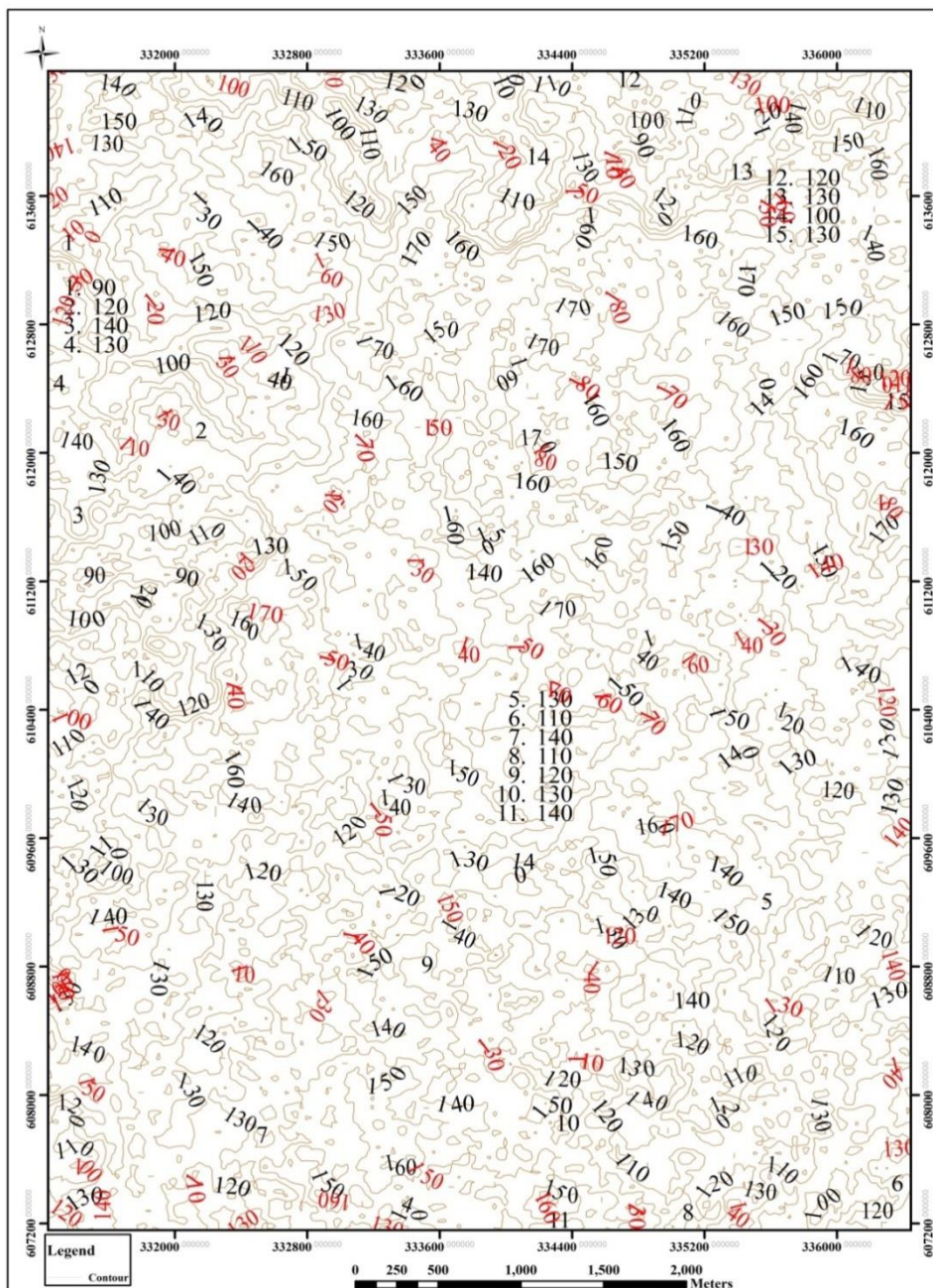
Figure 5. The Contour of Umuahia Urban showing undulating terrain The Impact of Reclamation for a Sustainable Infrastructural Development on Food Security in Umuahia Urban Using Geo-Spatial Technology (10760) Source: The researchers' Analysis (2020).
