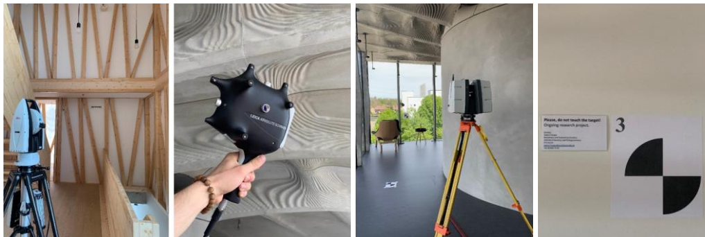
Figure 2: LT Leica AT960-XR during measurements (far left), Leica Absolute Scanner LAS during use (left), LS Leica P50 during scanning process (right), and laser scanning target installed in the SmartSlab module (far right).
