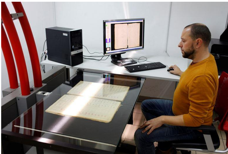
Illustration 3: Digitisation of parcels on the so-called book scanner by using a glass plate (Zeutschel optical scanner Q1; photograph: Boštjan Pucelj).
