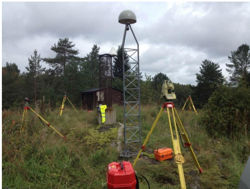
Figure 4. Control measurements at the Joensuu GNSS stations. Tripods are on survey markers founded on bedrock. New FinnRef station JOE2 is in the front and old JOEN in the back.
