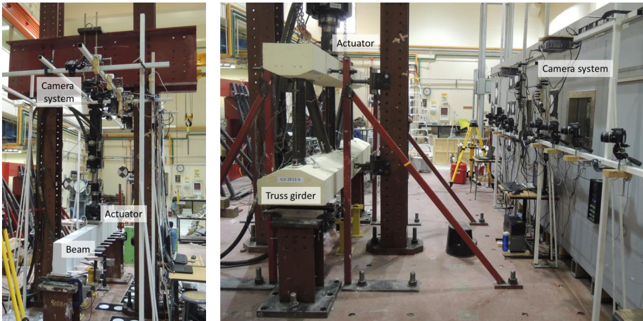
Figure 6: Suspended camera system setup (also showing the hydraulic actuator and the concrete beam specimen) (a); upright camera system setup (also showing the hydraulic actuator and the truss girder specimen) (b)
