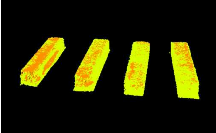
Figure 4: HDS3000 intensity return values for the four concrete samples
