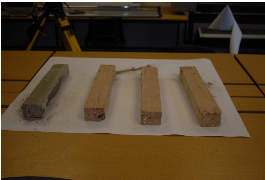
Figure 3: Four concrete samples, the three to the right have been heated to 990°C, the one on the far left has been kept at room temperature
