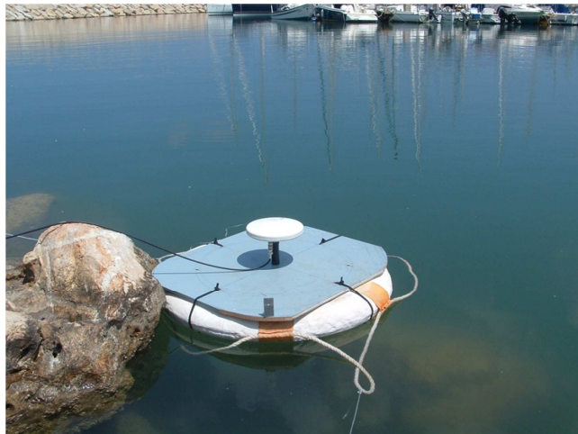
Fig. 2 – The GNSS buoy that was used during the experiment
