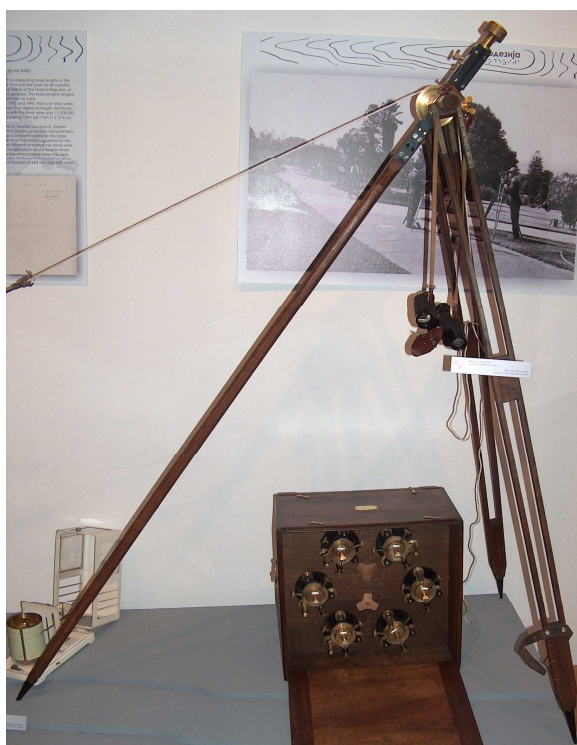
Fig. 7: The tripod for stretching the wires, with the set of supports in the box
