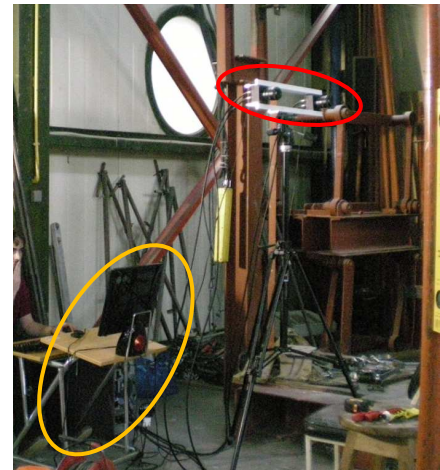
Figure 3: Photo of the cameras setup. The base of the two cameras on a stable tripod, and the PC for the operation control and the storage of the image frames
