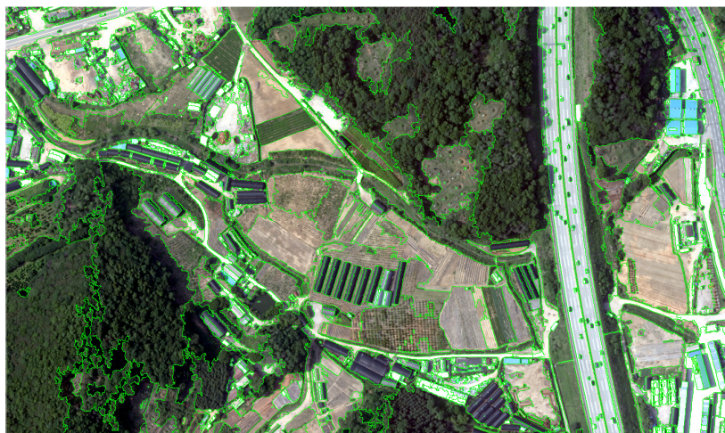
Figure 3. Third step of the feature extraction: Merge Segments
