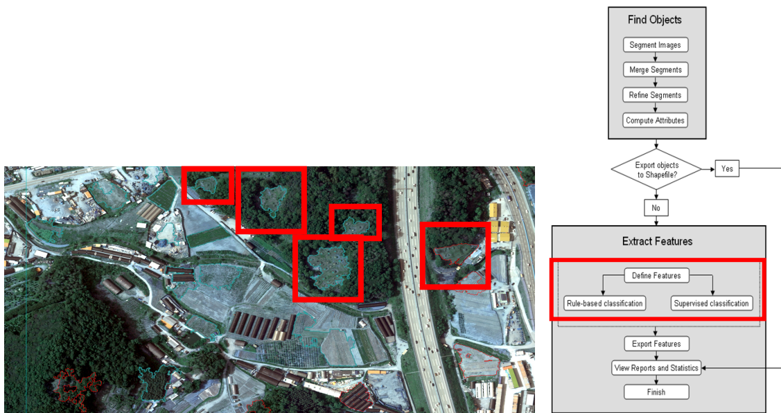
Figure 5. Fifth step of the feature extraction: Rule-based or Supervised Classification
