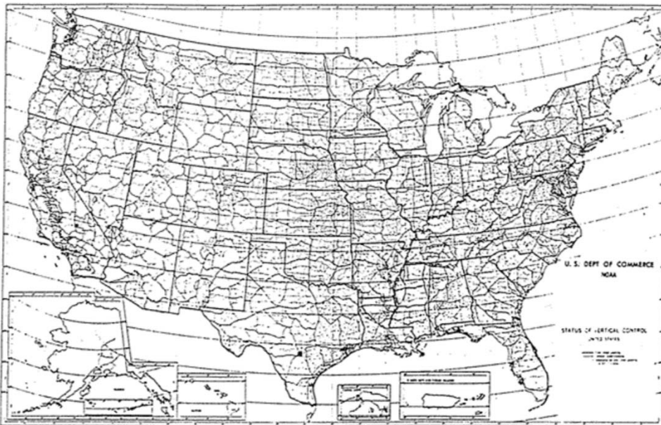
Figure 3. Vertical control used in 1988 adjustment.
