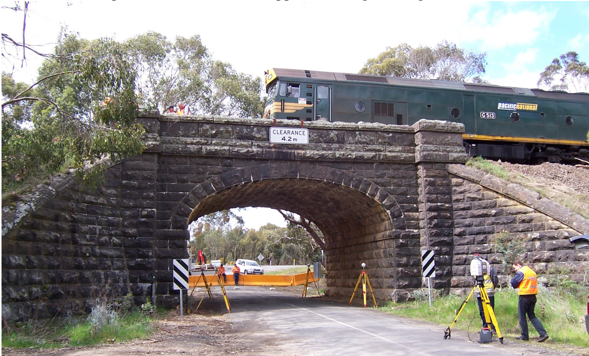
Fig 10: Load test on blue stone bridge.
