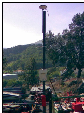
Leica GX1230GG receiver installed on the deck
