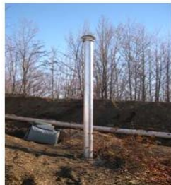
Example of GPS benchmark – periodic survey fixed in the soil for 1.5-2 m
