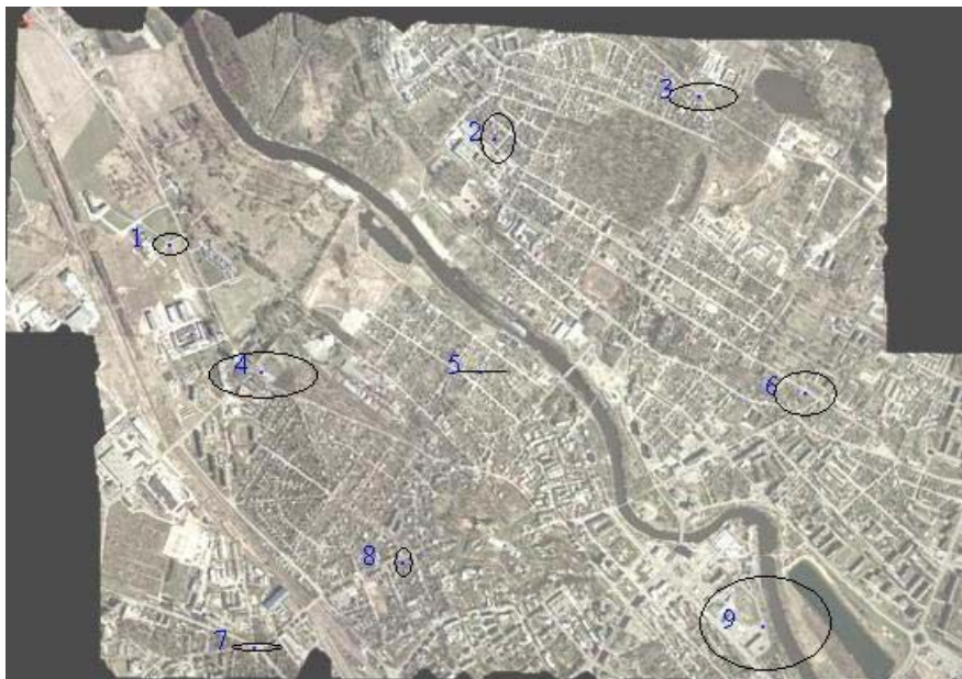
Fig 6. Location of control points and differences on the orthophotomosaic
