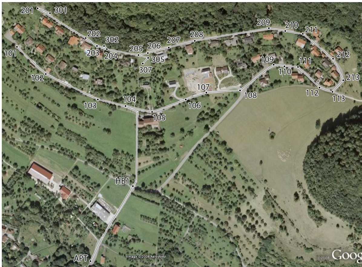
Figure 4: Height network, installed at the slope of the study area
