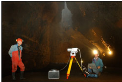
Fig 2. A laser-scanner in a cave (Picture copyright Yorkshire Post Newspapers)
