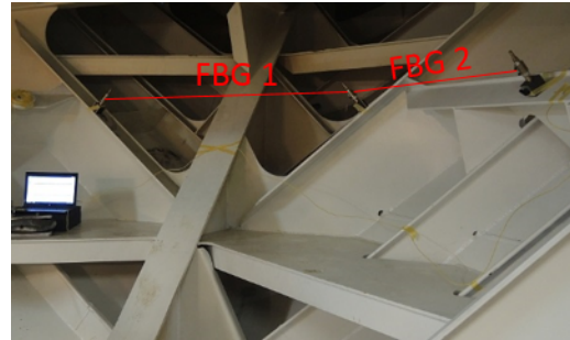
Figure 3. Location of the FBG sensors in the bow
