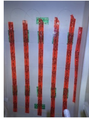
Figure 6. Commercial available strain chain (HBM, 2019) (top); FBG sensor arrangement (middle); final mounting setup (bottom)
