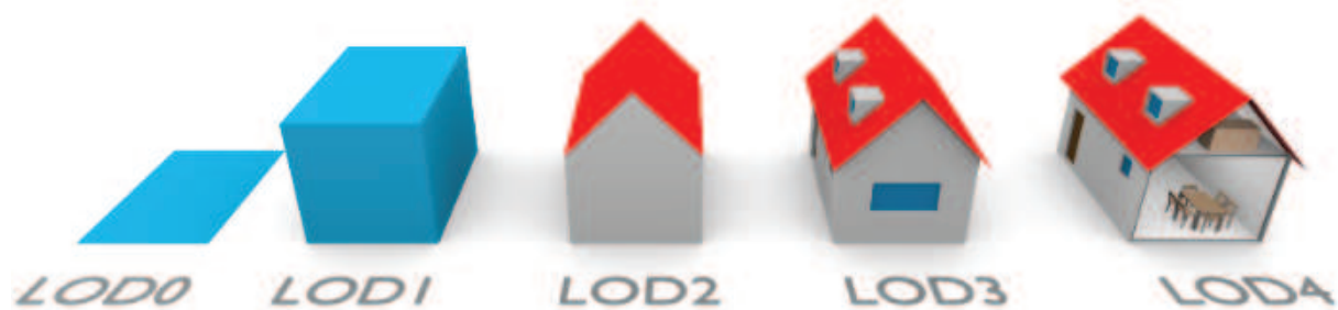
Figure 5. The five LODs of CityGML 2.0. The geometric detail and semantic complexity increase, ending with LOD4 containing indoor features (Biljecki et al, 2016)
