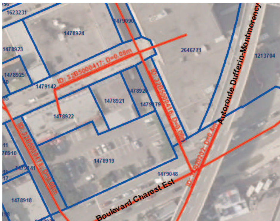
Figure 1. Visualization of communication cables (orange) with land parcels (blue) and the name of streets superimposed over orthophotography
