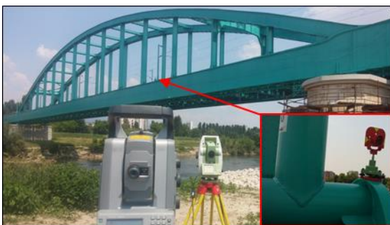
Fig. 3 Position of RTS instruments and reflector.
