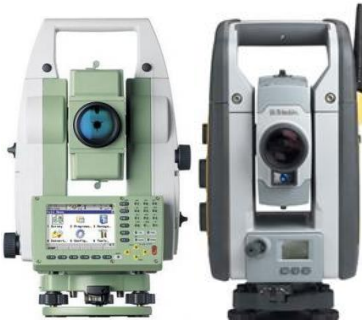
Fig. 5 Leica TPS 1201 and Trimble S8.
