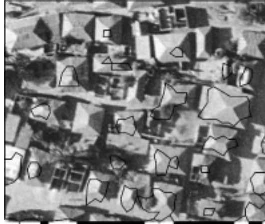
Fig. 4 Intermediate processing stage showing detected blob edges
