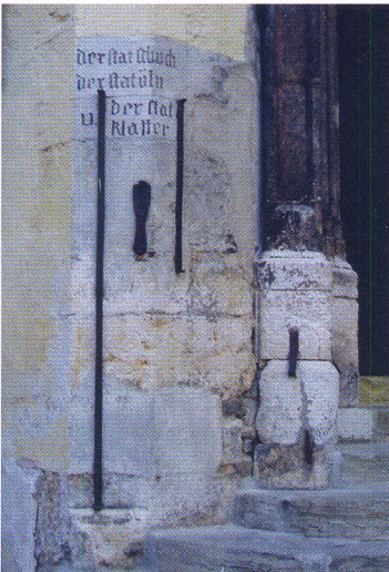
Above: Ruth Adams discovered these reference marks from ancient times in Regensburg. They show foot, yard and fathom rules fixed to the market place wall.
