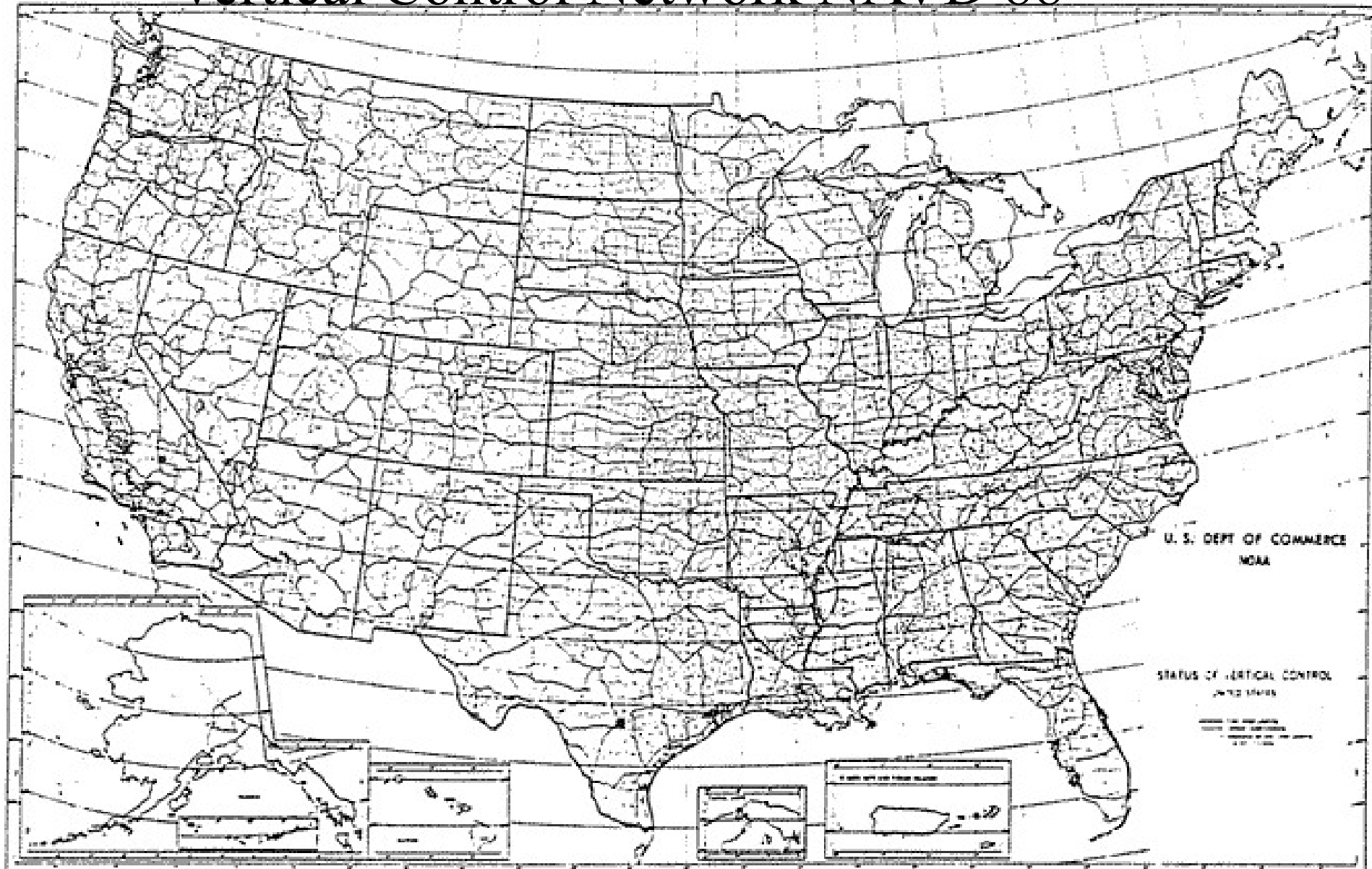
Figure 3. Vertical control used in 1988 adjustment.
