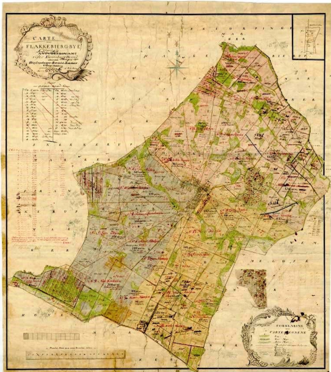
Figure 3. Another enclosure solution is the so-called star-enclosure where the buildings remain in the village and the land is allocated from there in a kind of star formation. This original map shows such an enclosure design. (Courtesy of the Danish Geodata Agency).
