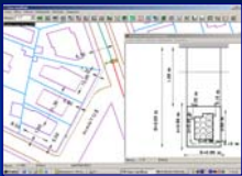
Fig.7: Main window: The piping level is active Secondary window: Cross-section dimensioned
